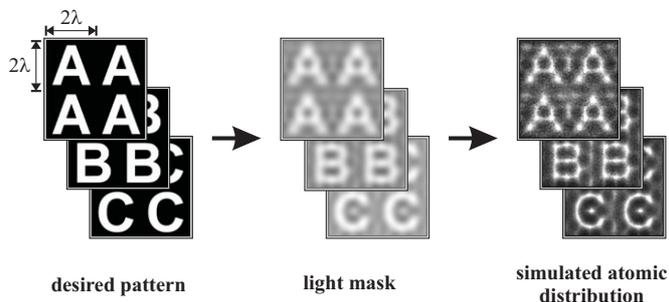
**Figure 4.** ANF generation of letters from a superposition of 24 standing wave light fields with different frequencies. Computer simulation from [20]
