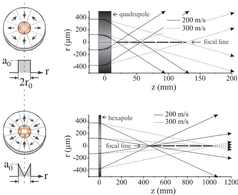
**Figure 6.** Magnetic 4-poles and 6-poles and their concentrating action on atomic trajectories. The 4-pole is the equivalent of an optical axicon, where parallel incoming trajectories of mono-velocity atoms are bent into a series of parallel outgoing trajectories. The 6-pole is equivalent to the optical lens and
