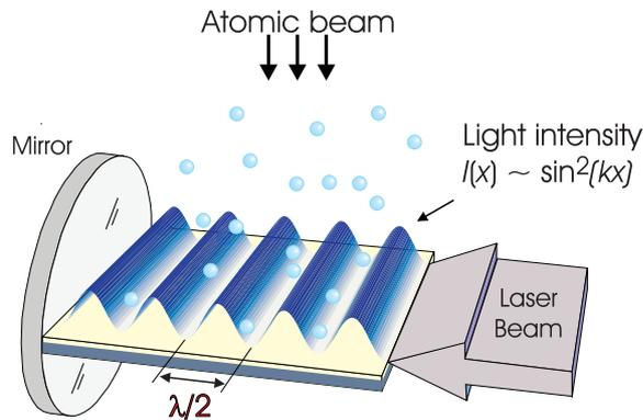
**Figure 2.** The well known concept of atom lithography: An atomic beam travelling through a standing wave light field towards a substrate is focused into narrow lines. If the laser is blue (red) detuned from the optical transition frequency optical dipole forces are exerted towards the nodes (antinodes) of the light field.
